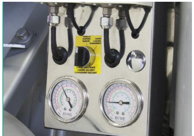
High- and low-pressure gage monitoring the cooling system
