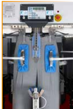
Pleat clamps with pre-steaming function.
